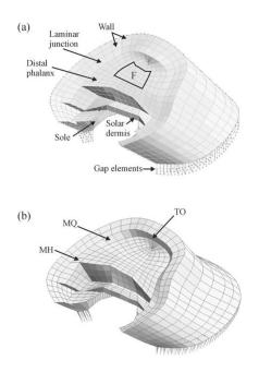
Figure 1: (a) A complete finite-element model with component layers and structures labeled, representing the unloaded hoof. (b) The same model showing global hoof capsule deformation (exaggerated) representing the loaded hoof. Reprinted from Thomason JJ, Mclinchey HL, Faramarzi B et al. Mechanical behavior and quantitative morphology of the equine laminar junction. 2005, The Anat Rec 2005; Part A, 283A: 366-379.
