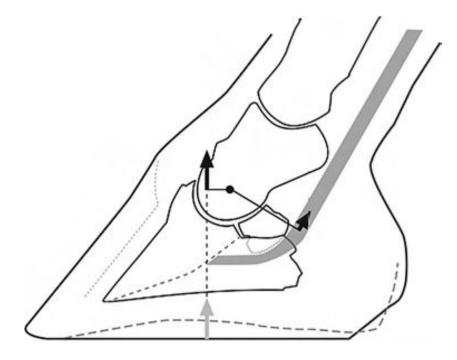
Figure 3: At rest, the ground reaction force (gray arrow) is dorsal to the center of rotation of the distal interphalangeal joint. As such, it creates an extensor moment that is opposed by an equal and opposite moment, the flexor moment, generated by the force in the deep digital flexor tendon so that the foot is stationary. Reprinted from Parks AH. Aspects of functional anatomy of the distal limb, in AAEP proceedings 2012.
